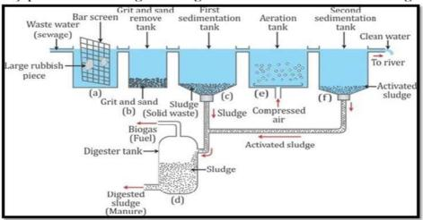
In primary treatment, floating debris is removed by sequential filtration. Grit (soil and small pebbles) are removed by sedimentation.
