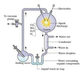
Miller created similar condition of temperature and pressure in laboratory scale. He created electric discharge in a flask containing CH4, H2 and NH3 and water vapour at 8000C.
